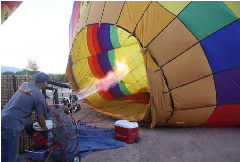
Figure 2: Crew Using Burner to Fill Balloon with Hot Air. Authored by: mnchilemom License: CC BY 2.0
